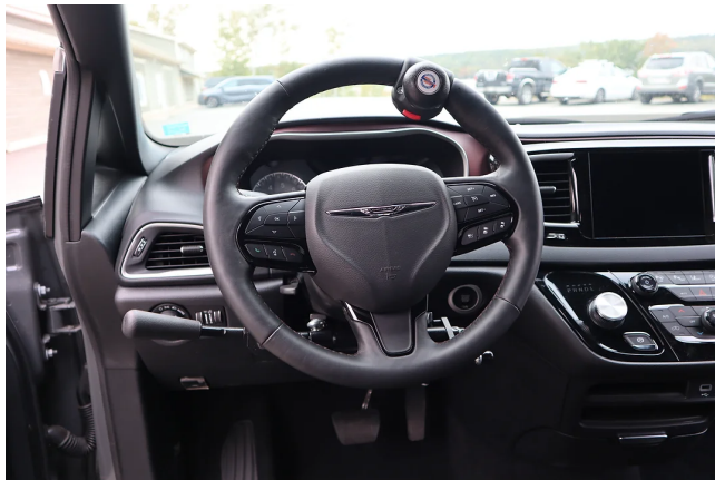
Figure 9: SureGrip's Push/Right Angle. This product only comes as a horizontal bar, whereas the other categories have the option of a vertical bar too.
