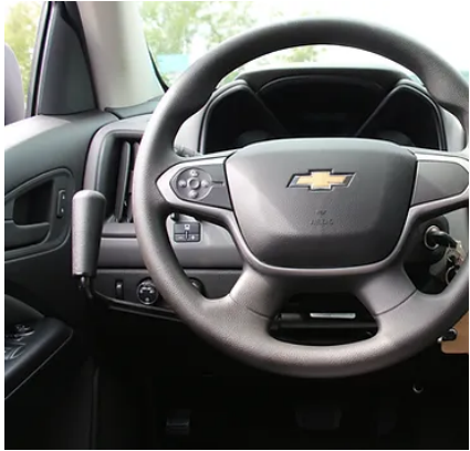
Figure 8: SureGrip's Push/Rock hand controls. This one uses a vertical handlebar, however it can also come horizontally depending on the company.
