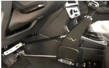
Figure 17: Image of the installation and placement of YANGG Hand Control product
