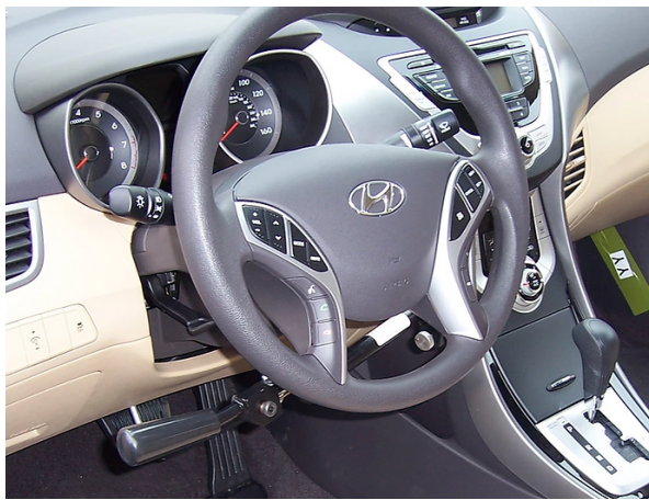
Figure 7: SureGrip's Push/pull hand controls. This particular one is installed on the left of the steering wheel, which is a very seamless addition to the vehicle.
