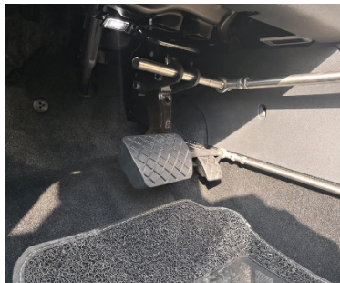
Figure 14: Figure 14 displays the installation of the floor accelerator pedal.
