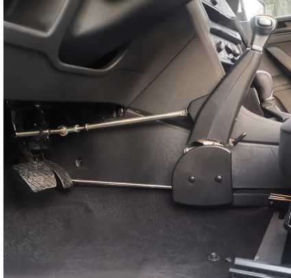
Figure 13: Figure 13 displays the product installation process. It does not require drilling. It can be directly fixed to the driver's seat rail.
