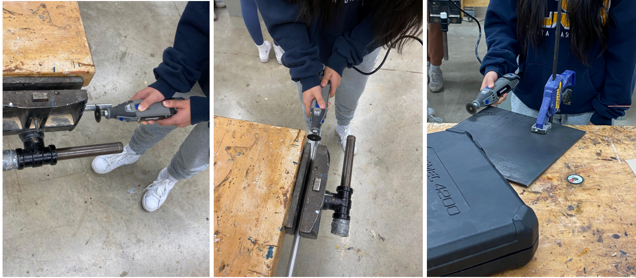
Figure 5 The metal sheet was initially cut with a small Dremel.
