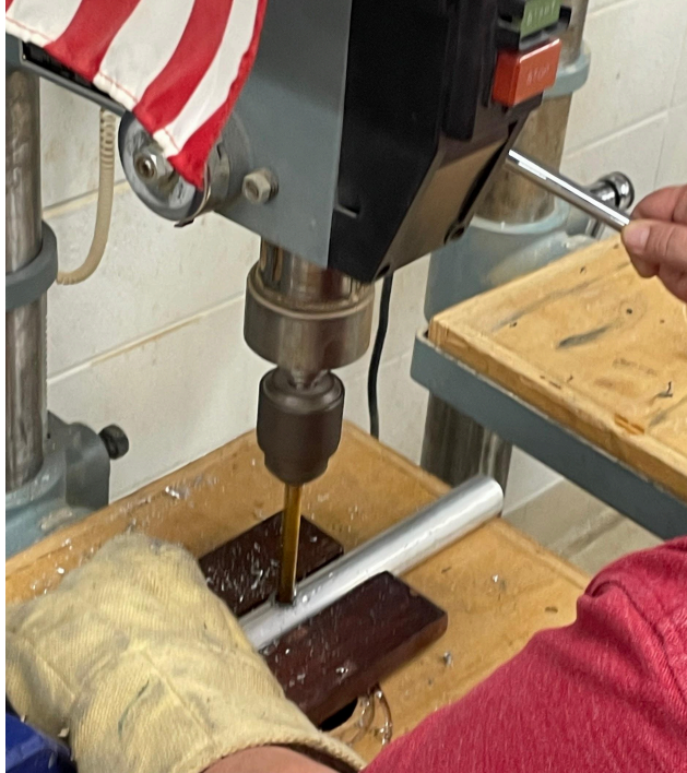
Figure 7 A hole is drilled into the solid rod with adult assistance.
