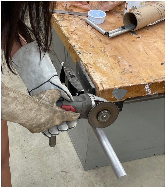
Figure 8 The solid rod is cut using the larger blade.
